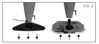
3. Insert the black connector of the H2O Dual Buff<sup>™</sup> unit into the H2O HD<sup>™</sup> steam mop body, then insert and tighten the screw. Note: use the same mop head screw removed from the H2O HD<sup>™</sup> body in step 2 above. Attach the H2O<sup>™</sup> HD Mop Head, then insert and tighten the provided screw into the hole on the back (screwdriver not included).
