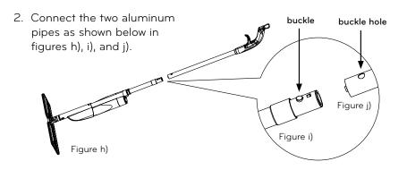
NOTE: The buckle hole on the upper aluminum pipe should be aligned with the buckle on the bottom aluminum pipe when connecting. Make sure that the buckle clicks into the buckle hole for secure assembly.  Insert the eActivator into the eActivator Holder as shown in figures k), l) and m) below. Then, turn eActivator locking mechanism to secure the eActivator in place, see figure m).
